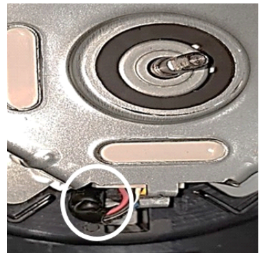
(b) Reappearance of a defect by cable
