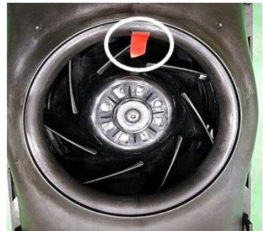
(a) Reappearance of a defect by tape
